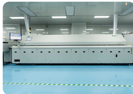
12-Zone Nitrogen Vacuum Reflow Oven
